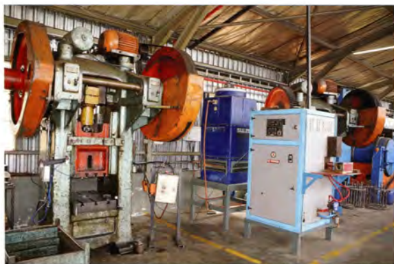
Robb and Carter have recently purchased two 150 ton eccentric presses, one 120 ton hydraulic press and a 120kW LH Power induction furnace. The company is now capable of manufacturing its own dies, as they do with all their jigs and fixtures, and now have a simple but effective forge in operation
