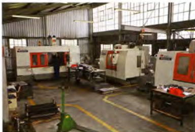
A cell of Victor Fortune machines including the latest addition, a Victor VC205 CNC machining center
