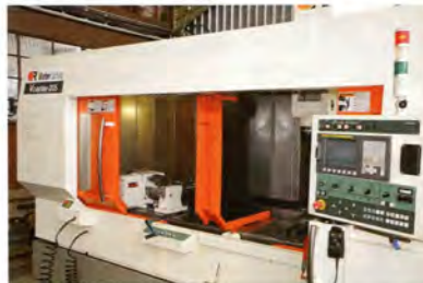
The Victor VC205 CNC machining center has a two metre bed and comes with a removable partition that allows Robb and Carter to load/unload a component on one side of the table while another component is being machined on the other side of the table
