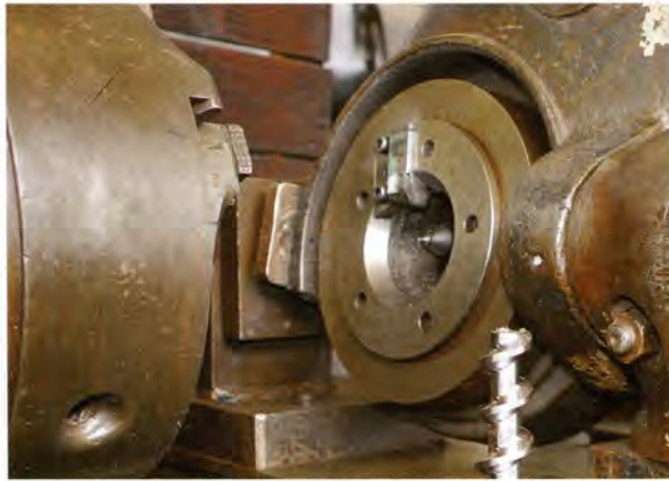
Robb and Carter was one of the first engineering companies in South Africa to make use of thread whirling and still offer the service today
