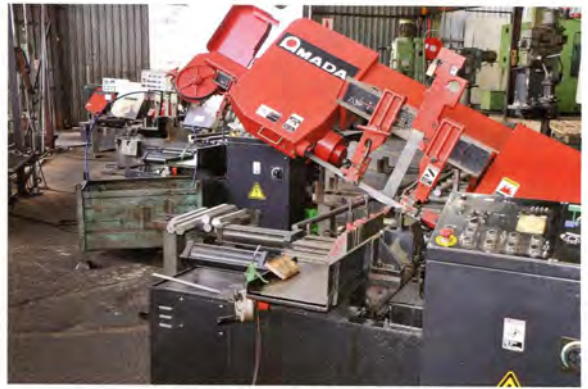
Robb and Carter have four bandsaws that are cutting bar to size
